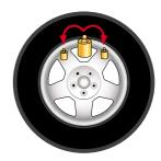
"Hidden Weight" program (in Alu P) which subdivides the adhesive weight for the outside into two equivalent weights positioned behind the spokes of the rim
